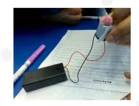
Tape the battery to the inside of the cup, with the wires facing out. Tape the motor to the side of the cup.
